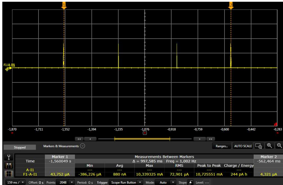
Figure 5. Measuring Standby Current During Connection (CC26x0)
