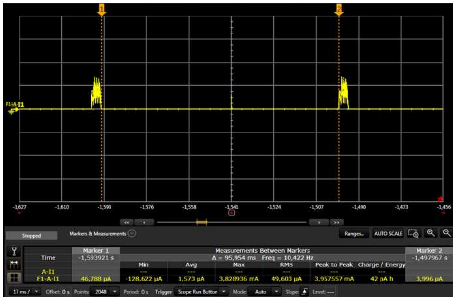
Figure 3. Measuring Standby Current During Advertisement (CC26x0)
